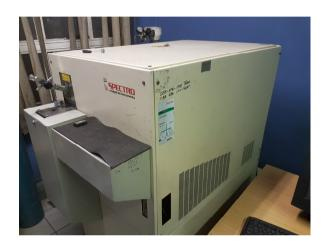
Some of the latest technology is fully utilized by Hi Alloy Castings. Included in this is the emission spectrometer and Magma simulation software which is currently only used by a few foundries in the country.
