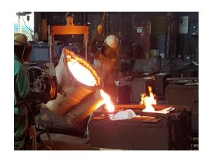
The casting process is carefully monitored to ensure that the exact temperatures are reached so that high quality castings are produced with little or no rejects. Each casting has a batch number to allow for traceability.
