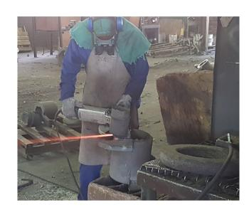
When the castings temperature have dropped to the required standard, they are knocked out and fettled to the final product.
